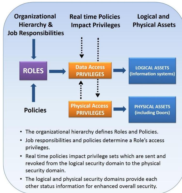
**Figure One<sup>4</sup>** : Physical/Logical Access Interoperability (Conceptual).
