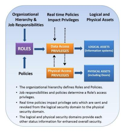
**Figure One**<sup>4</sup>: Physical/Logical Access Interoperability (Conceptual).
